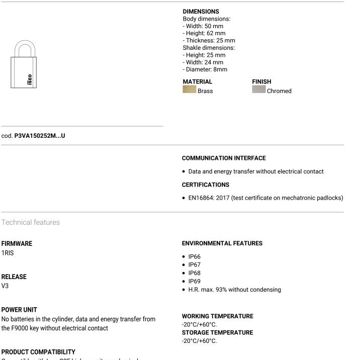
Compatible with Iseo CSF high security mechanical cylinders.
